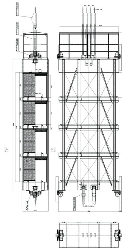
the supporting frame is filled up with steel sheets (load boards). If necessary, the operating weight can be altered by adding or removing of steel sheets. Counter-weight is guided in steel shaft guides through wheel guide and fixed guides. The installation of the upper and lower brackets is similar to the one for skips and cages.
